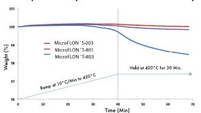
Increased Temperature by 10°C/min up to 420°C, then held temperature at 420°C for 30min
